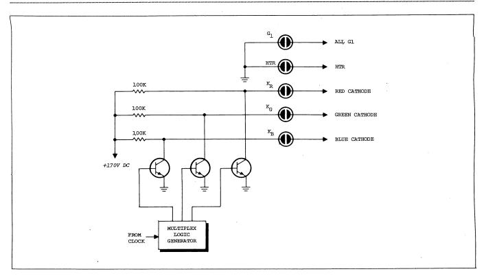
Fig. 9. Model 490 leakage test circuit (simplified).
